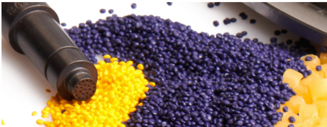
Example of a multi-hole nozzle with 22 holes each \varnothing 0,4 mm
